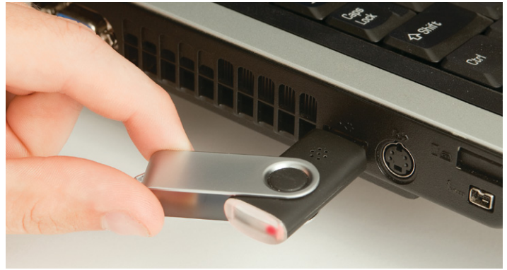
Figure 3 – The Indoor Air Monitor plugs into the USB port of a laptop or PC to indicate whether classroom air is polluted.
