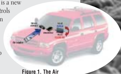
Figure 1. The Air Classification Module, mounted in the air intake of the HVAC system, protects occupants of a vehicle by automatically closing the fresh air inlet door when the sensor detects noxious gases and VOCs.
